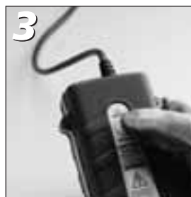
3 Press and hold operating switch and wait for the ignition
