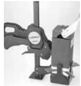
Step 4 Close the cover and ignite with flint ignitor. Open the mould after 10 seconds
