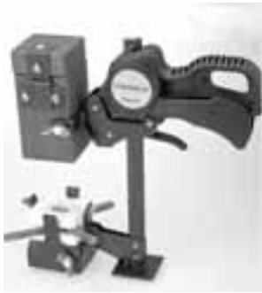
Step 1 Layer batting and variable conductor sizes to be welded into dry mould
